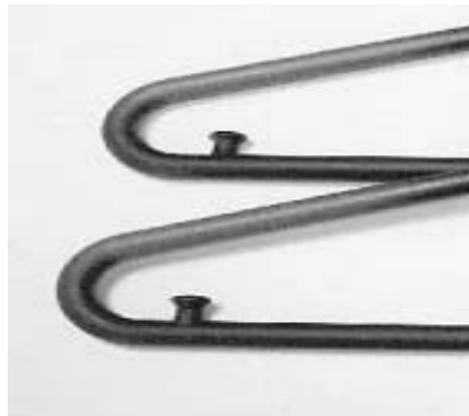
Figure 10.16 Marbling effect on a moulding
