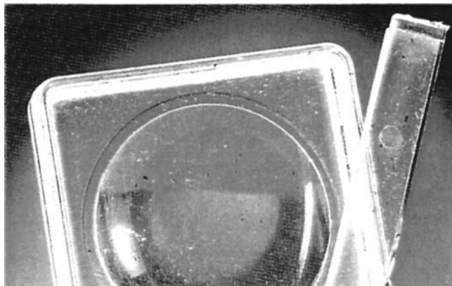
Figure 9.39 Dark spots due to thermal damage
